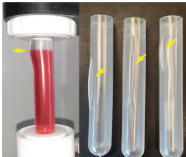
**SOLUTION:** Remove all 'restrictions' from the flowpath that can result in a pressure buildup. For this, e.g. remove flow restrictors and/or replace tubing with a small inner diameter by tubing with a large inner diameter.
