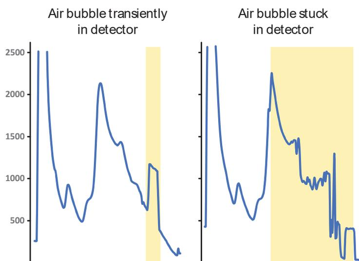
**SOLUTION:** Wash detector with warm water (optional: mild detergent solution instead of water) to remove contaminations that facilitate trapping of bubbles. Fractionate gradients at high flow rates (>2ml/min) to flush bubbles through the flow cell of the UV detector.
